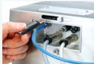
Built-in label creation software means you can create code formats on the line. Alternatively, you can design them on a PC using **EasyDesign** or other compatible label creation packages, and transfer via USB or Ethernet.
